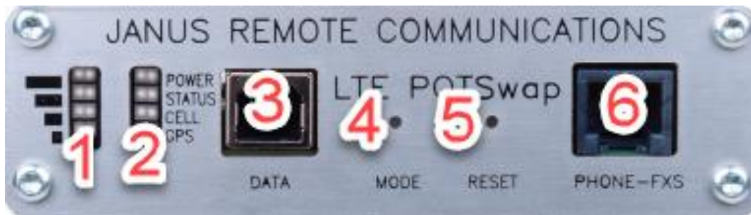
Figure 2. Front panel of the ETP-CI-4G-GSM Cellular Interface.
