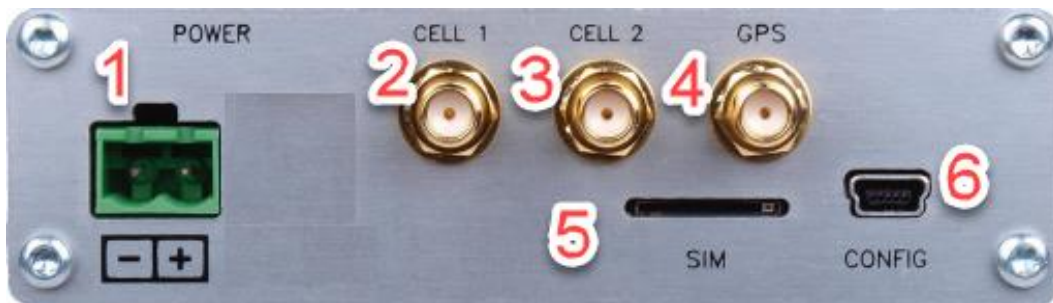
Figure 3. Rear panel of the ETP-CI-4G-GSM Cellular Interface.
