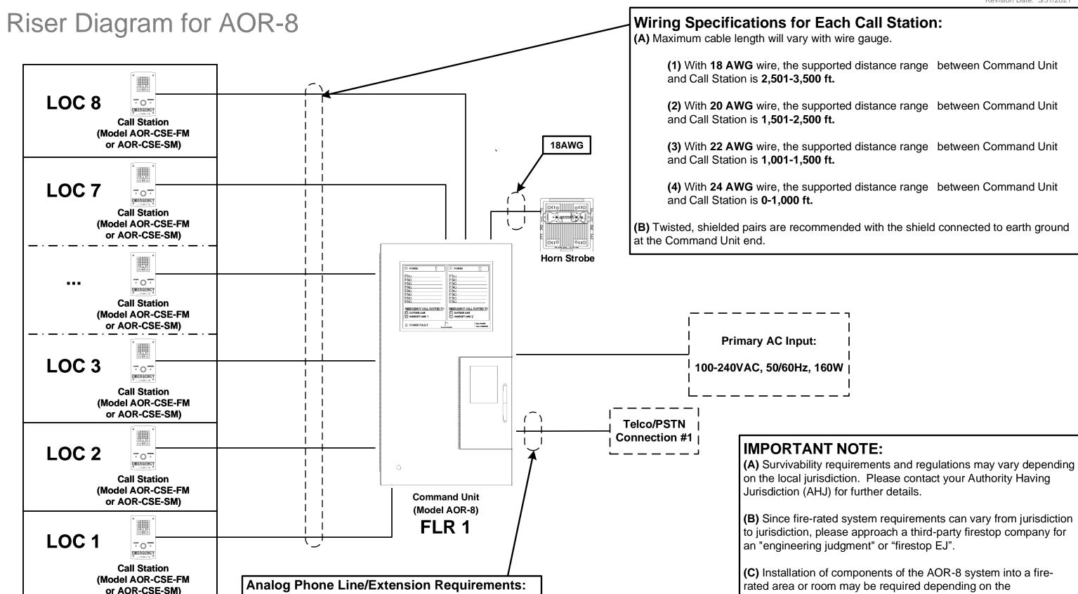
(A) Minimum of 24V talk battery and 20 mA off-hook loop current
